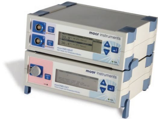
moorVMS-HEAT and moorVMS-OXY – setup showing skin heater and tissue oxygenation monitor.
