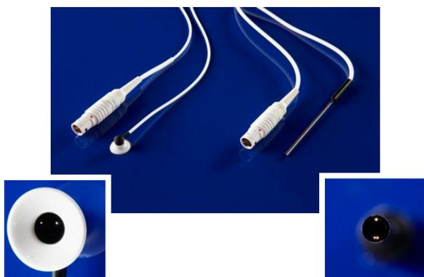
VP1-HP wide fibre separation (4mm) probe (left) and VP7BS-HP (right) with probe head inserts.
