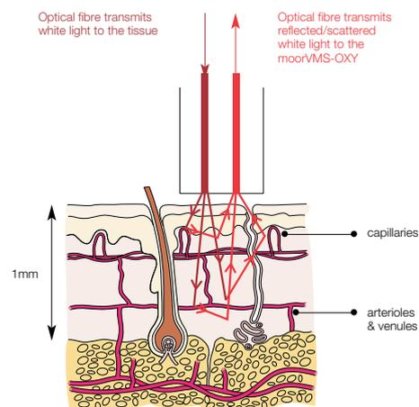
The moorVMS-OXY analyses the back scattered reflected light in the wavelength range of 500 to 650nm and calculates tissue oxygenation by matching the collected spectra to the absorption curves from known concentrations of oxygenated / deoxygenated haemoglobin.
